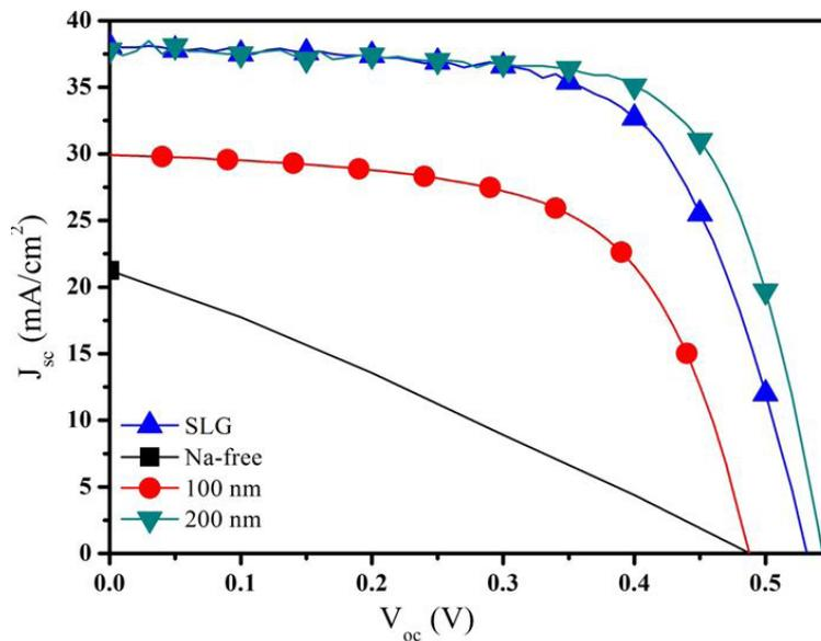
Figure 6: The I-V Characteristic of the solar cells with absorber layers deposited on SLG and different MoNa back contact thickness
