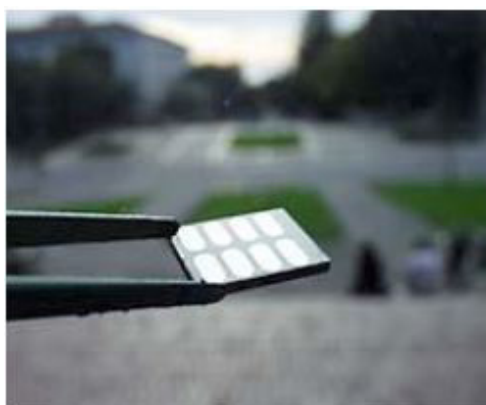
Figure 8: Picture of a solar cell, which utilizes nanorods to convert light into electricity [78,79]
