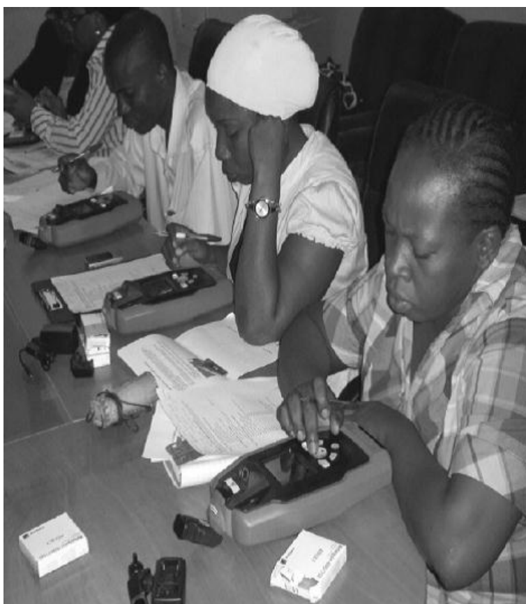
Figure 2: Thermo Scientific Incorporated Truscan™ handheld Raman Spectroscopy equipment (in use by NAFDAC counterfeit medicine inspectors) [17]
