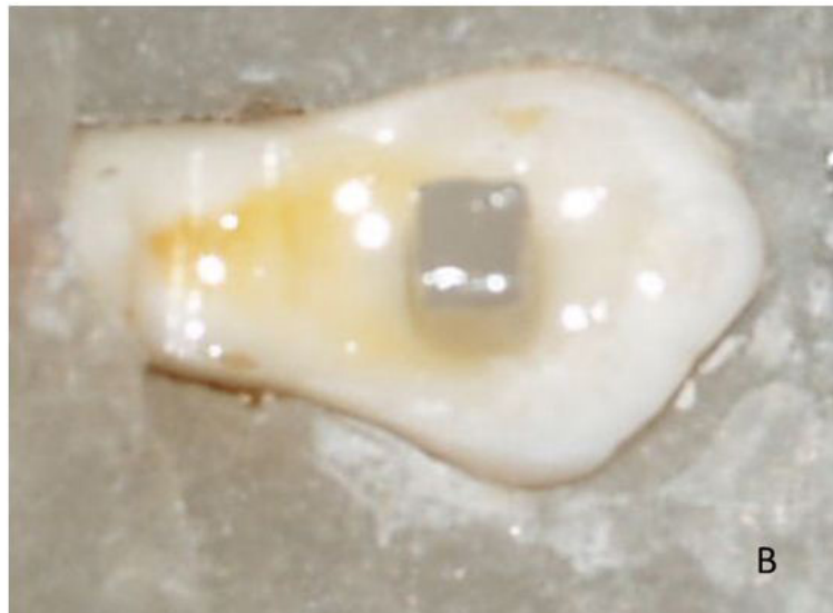
Figure 1: The teeth were embedded in acrylic resin with the buccal surface facing upward. A resin composite rod was built on the treated surface (A&B)
