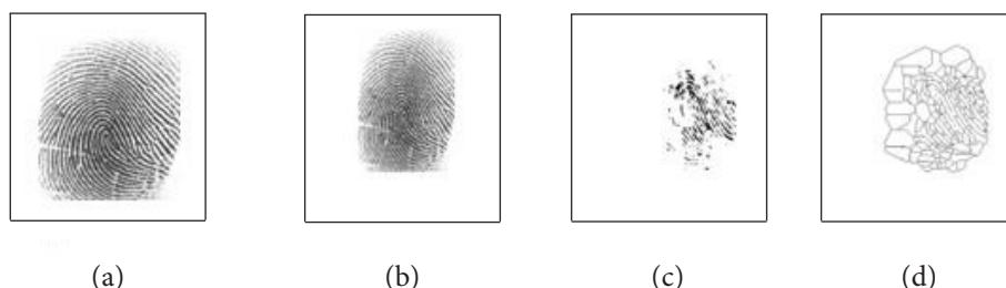
Figure 3: (a) is the chosen fingerprint from FVC2004 fingerprint database DB1. Fi. (b) is the filtered output by using Gabor filter. (c) is binary output of picture received from photo processing. (d) is image after Morphological operation the use of the ‘skinny’ recognized thinning of photo
